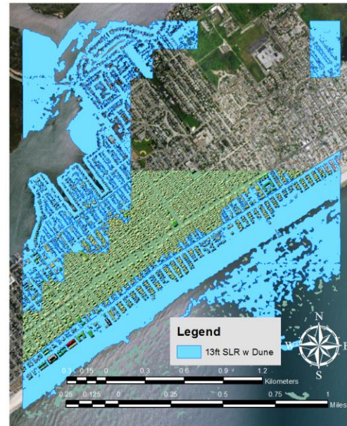
Figure 16b. Inundation simulations at 8.43ft and 13ft SLR on the 2012 Post-Sandy DEM either with or without a dune (4-Neighbor Model)
