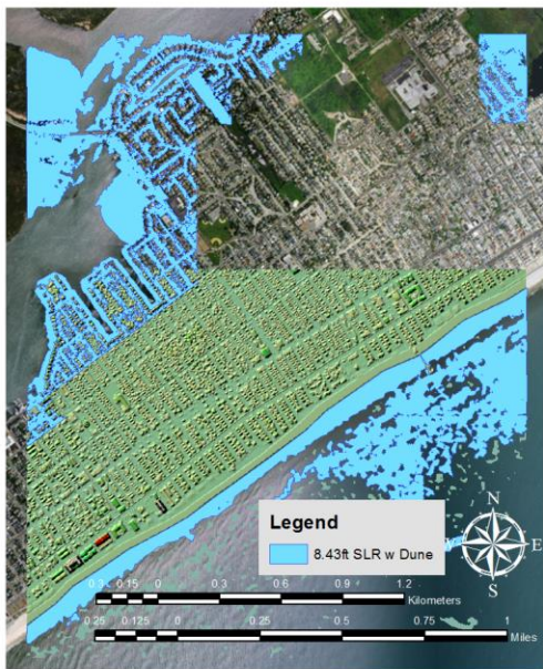
Figure 16b. Inundation simulations at 8.43ft and 13ft SLR on the 2012 Post-Sandy DEM either with or without a dune (4-Neighbor Model)
